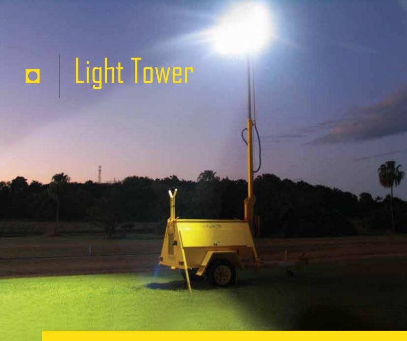
ITTS model LT4000 L light tower provides mobile trailer mounted flood lightning for nighttime maintenance, construction, mining and emergency work. It consists of a trailer with diesel powered 5KW generator and a 30 foot cable actuated tower with four 100 watt flood light fixtures. It is ideally suited for heavy duty use and is built to meet the following specifications.
